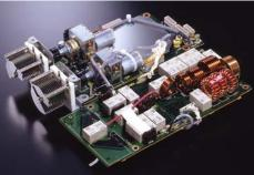
100-Watt Automatic Antenna Tuner
